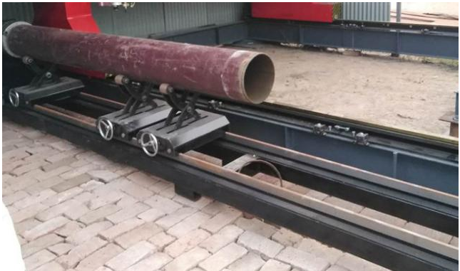
13. Pipe holder and ground track rail
